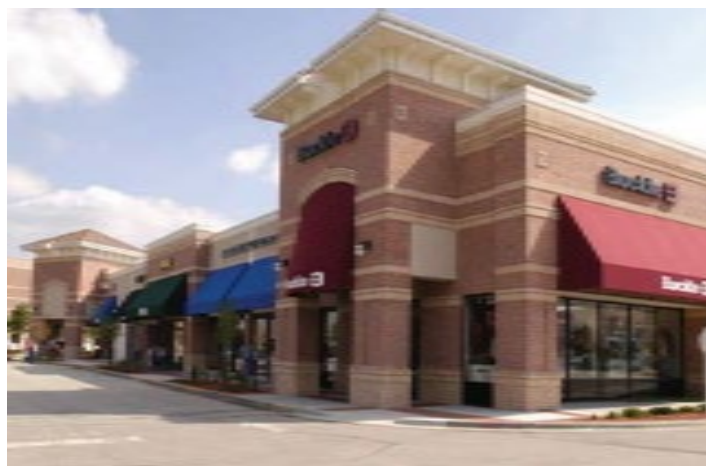
Figure C2.2: Combined vertical articulation and modulation minimize the appearance of a long, massive wall.
